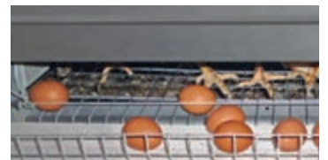
EggSaver in lowered position → the eggs are slowed down carefully
