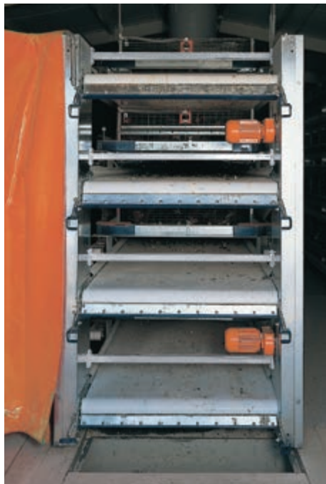
Manure removal end set with manure chute
